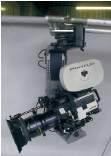
Above: Mehran Salamanti of Hot Gears designed and motorized the Lamdahead for intense sequences in Spider-Man 2 and National Treasure . Right and Below: Chapman-Leonard's new Amphibian three-axis remote head is not only waterproof, but can also go from land use to underwater without any additional housing for the head.
