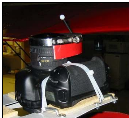
GLAB Designed Light Probe System Mounted on Pitts Biplane
